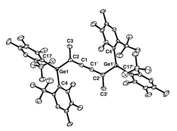
Fig. 4. Molecule of 7 in the crystal (hydrogen atoms omitted). Ellipsoids are drawn at 50% probability. Selected bond lengths (pm) and bond angles (°): C(1)-C(1') 122.8(13), C(1)-C(2) 138.9(9), C(2)-C(3) 152.9(8), Ge(1)-C(2) 181.9(6), Ge(1)-C(4) 199.7(5), Ge(1)-C(17) 197.6(6) and Ge(1)-C(2)-C(1) 120.7(4), Ge(1)-C(2)-C(3) 121.4(5), C(1)-C(2)-C(3) 117.9(5).
